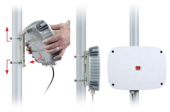
**6** Attach bracket to the mast using hose clamps. Clamps shall be as much to the outer edge of bracket, as possible.
