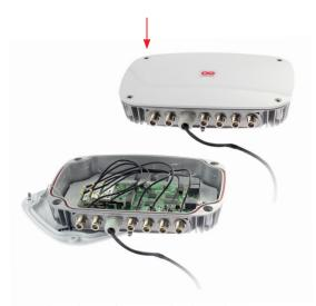
5 Close the enclosure and tighten the screws.
