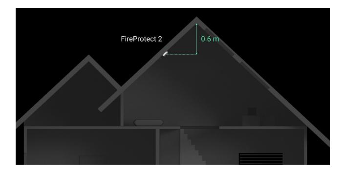
We do not recommend mounting the detector on a wall. This installation is acceptable if closely spaced beams or other obstacles interfere with the installation of the detector. Wall mounting is possible only if the detector is placed at a distance of 15–30 cm below the ceiling but above the doorways.
